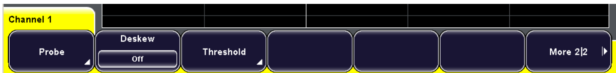
Fig. 5-2: Menu: "Probe" opens the submenu, "More" switches the menu pages
